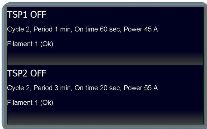
Figure 17. TSP Sublimation View Screen (no control buttons)
